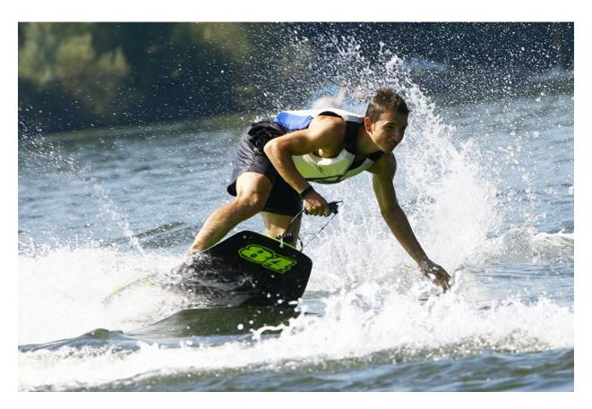
The Jet Surf gasoline tank has a 3-liter capacity, the top speed between their three models is 35 mph, and they weigh around 30 pounds. According to the company, there is no comparable engine in the world that has the same power-to-weight ratio. Additionally, the Jet Surf riders do not need special permits, which is great if you want to casually test one out on the waterfront wherever you may be visiting all over the world.
